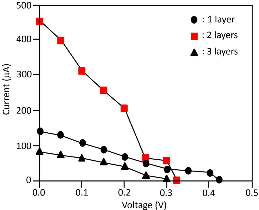
Figure 3 Effect of the number of active layers on the current–voltage characteristic of the solar cells: (circle) one layer, (square) two layers, and (triangle) three layers. An active layer is composed of  $\text{TiO}_2$  and graphite with Cu particles deposited in the space between  $\text{TiO}_2$  and graphite particles. The measurement was made under a xenon lamp with illumination intensity of  $37.38 \text{ W/m}^2$ .
