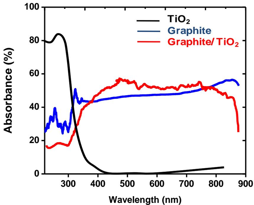
Figure 5. Ultraviolet–visible light characterization of pure TiO<sub>2</sub>, graphite and graphite/TiO<sub>2</sub> composite
