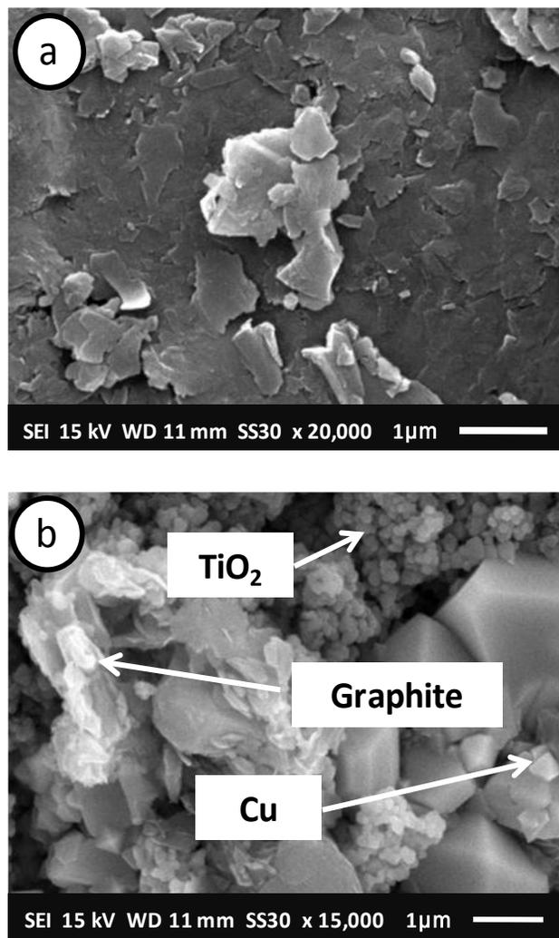
Figure 4. SEM images of (a) graphite and (b) Cu/graphite/TiO<sub>2</sub> film
