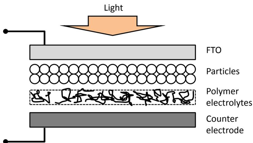
Figure 1. Schematic of solar cells investigated in this work. The solar cell is composed of a transparent conductive electrode (Fluorine-doped Tin Oxide), photon absorber particles, polymer electrolyte, and a counter electrode.
