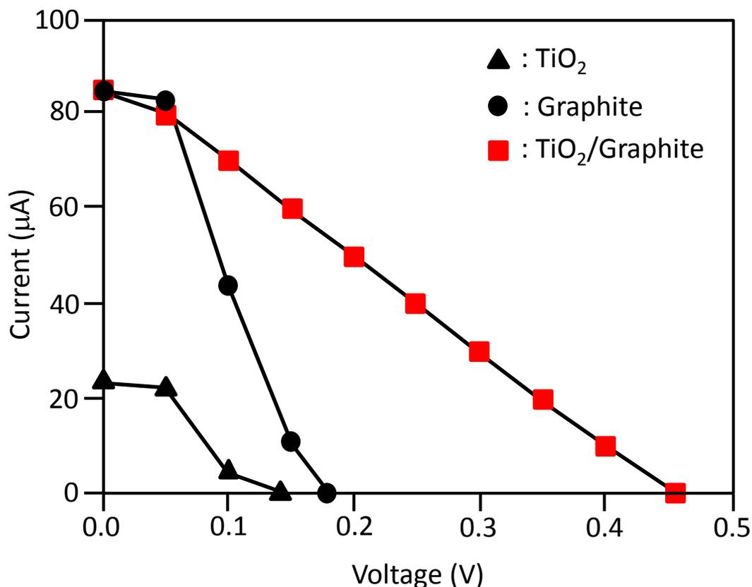
Figure 2 Current–voltage characteristics of solar cells containing an active layer of TiO<sub>2</sub> only (triangle), graphite only (circle) and a mixture of TiO<sub>2</sub>/graphite (square) with a graphite/TiO<sub>2</sub> ratio of 8 %w/w. The fill factors and efficiencies of the solar cells are 0.33 and 0.03%, 0.29 and 0.12%, and 0.26 and 0.27% for cells containing TiO<sub>2</sub> only, graphite only, and a mixture of TiO<sub>2</sub>/graphite, respectively.
