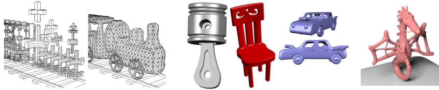
Figure 14: Implicit surface modeling. (left) A train defined by skeletal elements that define a blended surface [Bloomenthal and Wyvill 1990]. (middle) The ShapeShope system is a modeling-by-sketching tool that uses implicit surfaces as its shape representation [Schmidt et al. 2006]. (right) Later developments on the blending functions allowed for more precise modeling [Bernhardt et al. 2010].
