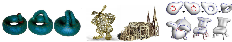
Figure 15: Interactive modeling of surface meshes. (left) A technique for modeling free-form 3D meshes of mutable topology [Welch and Witkin 1994]. (middle) The Topmod3d system is a specialized tool that helps users in modeling highly complex subdivision surfaces [Akleman et al. 2008]. (right) The FiberMesh system allows the user to change the topology of the shape with a single stroke. [Nealen et al. 2007].
