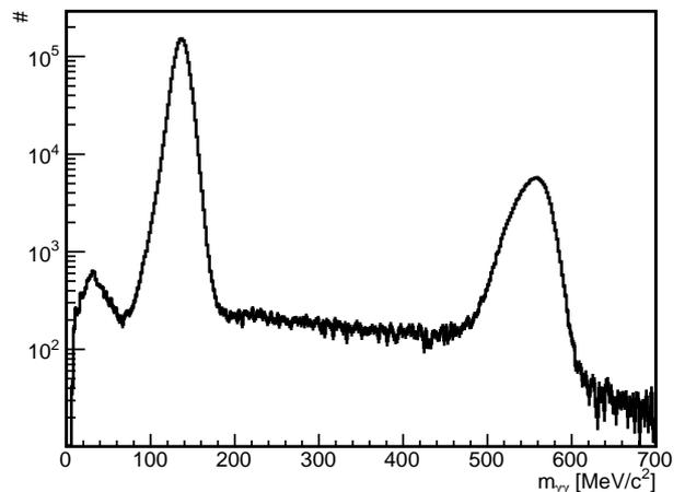
Figure 2: The invariant  $\gamma\gamma$  mass distribution for the butanol data, after all cuts discussed (see text) have been applied. The final data sample of  $p\pi^0$  events has a background contamination of less than 1%.
