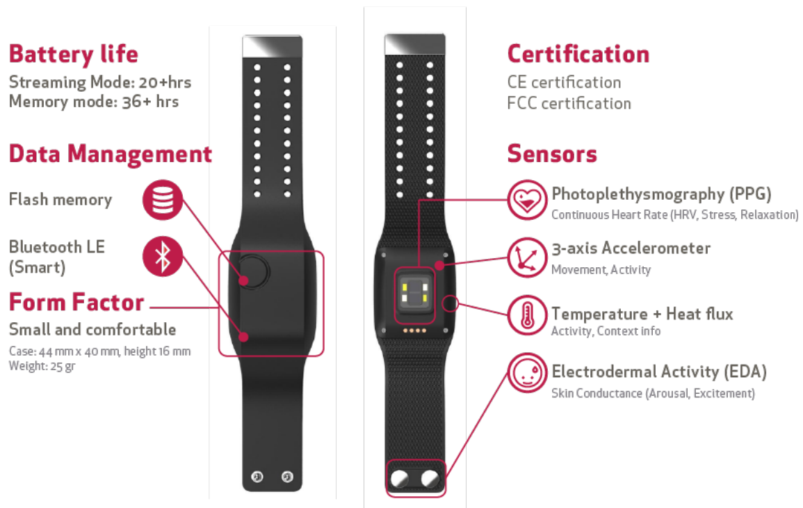
Figure 2. Smart watch sensors. [Source: internetmedicine.com]
