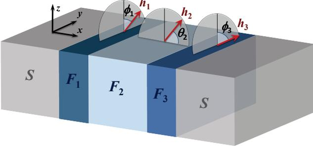
FIG. 1. Schematic of the  $SF_1F_2F_3S$  Josephson junction considered in this paper. A generic configuration is shown, described by the in-plane magnetization angles,  $\phi_i$ , and the out-of-plane angles,  $\theta_i$  ( $i = 1, 2, 3$ ). The ferromagnetic exchange field  $\mathbf{h}_i$  in each region is expressed as  $\mathbf{h}_i = h_i(\cos \theta_i, \sin \theta_i \sin \phi_i, \sin \theta_i \cos \phi_i)$ .
