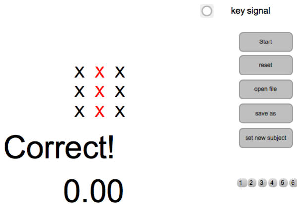
Fig. 2. The visual instruction screen presented to the users during the experiments programmed in MAX 6 [12]. The red × symbols inform about the pattern shape to be attended by a user in each SWLDA training experimental run.
