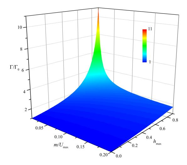
Figure 4. A quantitative diagram for toughening mechanisms of soft materials. The toughness enhancement ratio  $\Gamma/\Gamma_0$  as a function of  $h_{\text{max}}$  and  $m/U_{\text{max}}$ , calculated based on Eq. (3) and (8).
