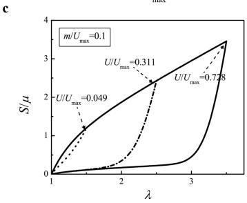
Figure 2. The modified Ogden-Roxburgh model for Mullins effect. (a) The relation between  $h_{\rm max}$  and r for a neo-Hookean material with Mullins effect under pure-shear deformation. (b) The calculated h as a function of  $U/U_{\rm max}$  for different values of  $m/U_{\rm max}$  for a neo-Hookean material with Mullins effect under pure-shear deformation. (c) The calculated stress-stretch hysteresis for a neo-Hookean material with Mullins effect under pure-shear deformation.
