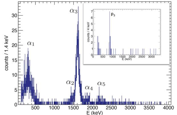
Figure 2: (Color online) Singles  $\alpha$  spectrum extracted from the Gas-Si telescope. The inset in the top right corner shows the DSSSD proton spectrum in coincidence with the low energy  $\alpha_1$  line.
