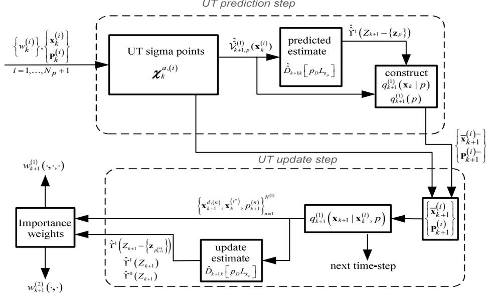
Figure 3. The schematic of how UT can be used to implement ACPHD filter and construct proposal distributions as well as computing importance weights.
