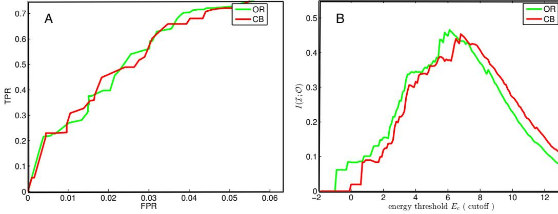
**Figure 3.** ROC and Information. (A) False positive rate ( $FPR$ ) vs. True Positive Rate ( $TPR$ ) when varying the energy cutoff  $E_c$ . (B) shows the mutual information  $I(\mathcal{I}; \mathcal{O})$  Eq. (18) between the input and output of the detectors as a function of the cutoff energy.
