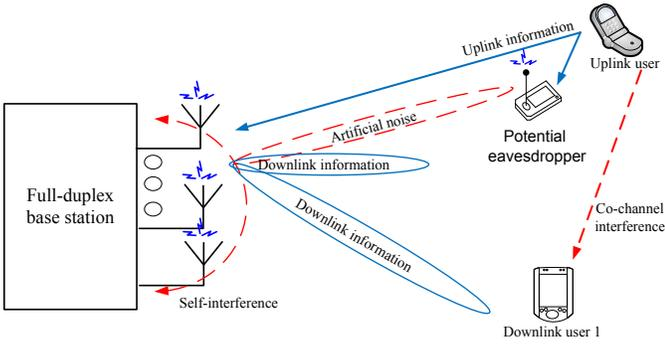
Fig. 1. Multiuser system model with an FD radio BS,  $K = 1$  HD downlink users,  $J = 1$  HD uplink users, and  $M = 1$  HD idle receivers (potential eavesdroppers). The BS is equipped with  $N$  antennas for facilitating secure simultaneous uplink and downlink communication.
