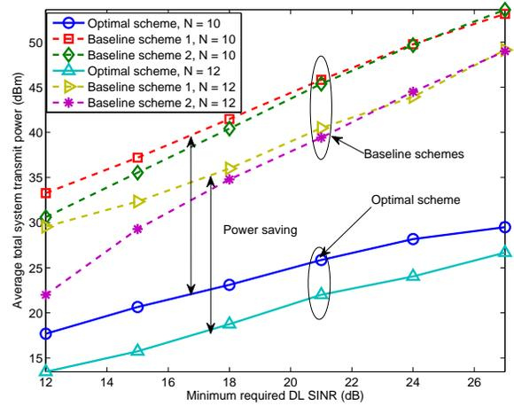
Fig. 2. Average total system transmit power (dBm) versus the minimum required DL SINR,  $\Gamma_{\text{req}}^{\text{DL}}$  (dB), for different resource allocation schemes. The double-sided arrows indicate the power saving enabled by the propose optimal resource allocation scheme.
