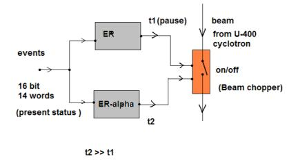
Fig.7. Schematics of the combined beam-stop real-time algorithm.
