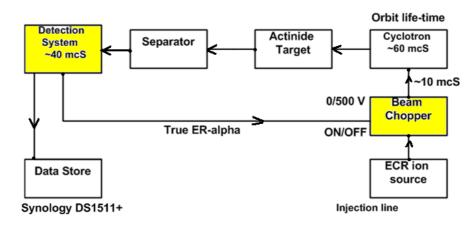
Fig. 1a. Block diagram of real-time process. Two key elements are shown in yellow color.
