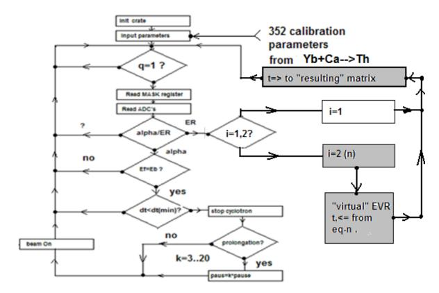
Fig.3. The flowchart of the modified process. Branch n >1 is in grey color.
