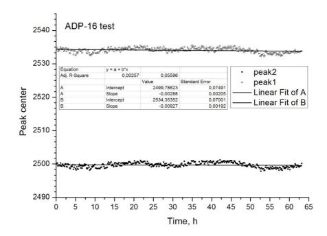
Fig. 8b Stability test for ADP-16(left peak in the 6a). Linear fit results are presented in the table within.
