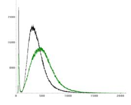
Fig.5a Typical shapes for EVR  $\Delta E$  signals (channels) measured with START and STOP proportional chambers. The pentane pressure value is equal to 1.6 Torr. Both anode biases are equal to +390 Volts. Both cathode biases are equal to -100 Volts. Reaction:  $^{nat}Yb + {}^{48}Ca \rightarrow ^{*}Th$ .
