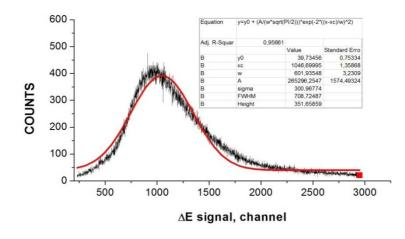
Fig.5b Gaussian fit of the ∆E signal for (200, 3000) range. Fit parameters are within the frame
