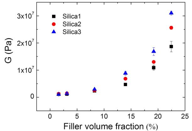
FIG. 2. Elastic modulus  $G$  versus filler volume fraction for the three types of silica. Black color is for Silica1, red for Silica2 and blue for Silica3. The Silica particle size decreases from Silica1 to Silica3.
