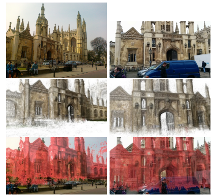
(e) Relocalization with unknown camera intrinsics: SLR with focal length 45mm (left), and iPhone 4S with focal length 35mm (right) compared to the dataset's camera which had a focal length of 30mm.
