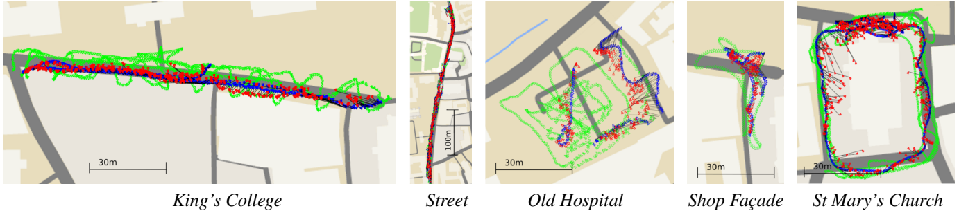
Figure 4: Map of dataset showing training frames (green), testing frames (blue) and their predicted camera pose (red). The testing sequences are distinct trajectories from the training sequences and each scene covers a very large spatial extent.
