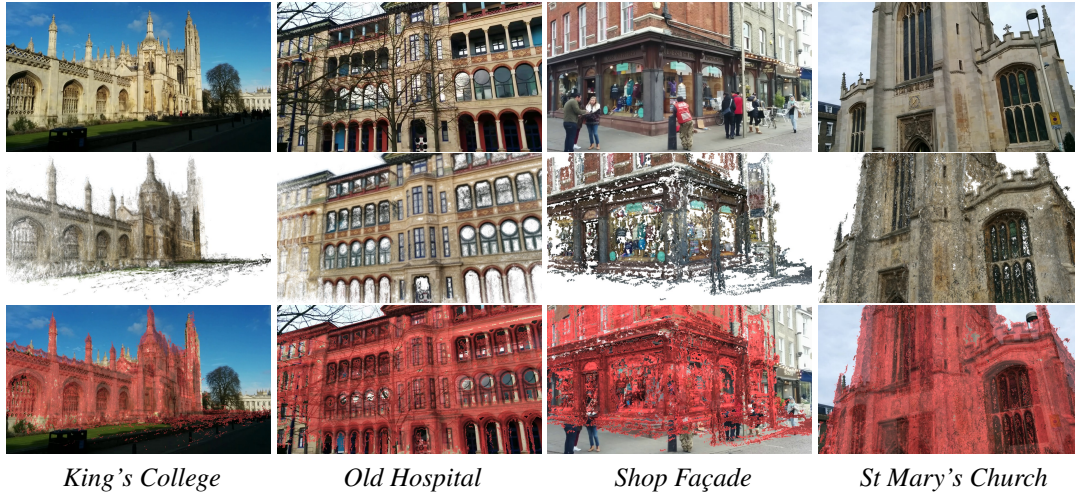
Figure 1: PoseNet: Convolutional neural network monocular camera relocalization. Relocalization results for an input image (top), the predicted camera pose of a visual reconstruction (middle), shown again overlaid in red on the original image (bottom). Our system relocalizes to within approximately 2m and 6^\circ for large outdoor scenes spanning 50,000m^2 . For an online demonstration, please see our project webpage: mi.eng.cam.ac.uk/projects/relocalisation/
