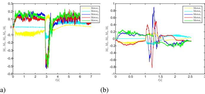
**FIGURE 18.** Percentage of the motor torques sent to the drives (a) the linear trajectory and (b) the circular trajectory
