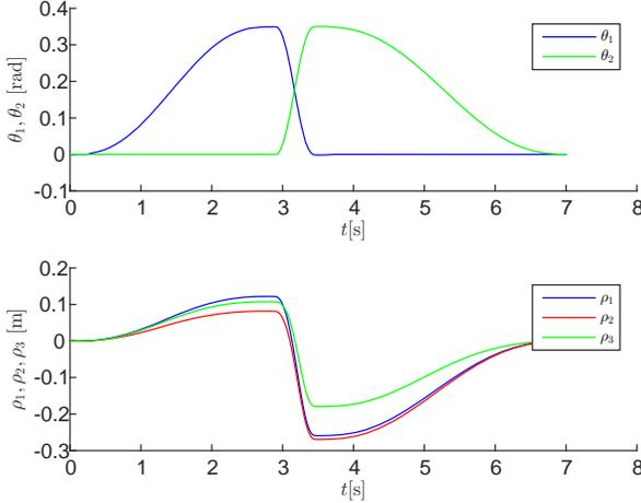
**FIGURE 8.** Joint values along the complete linear trajectory
