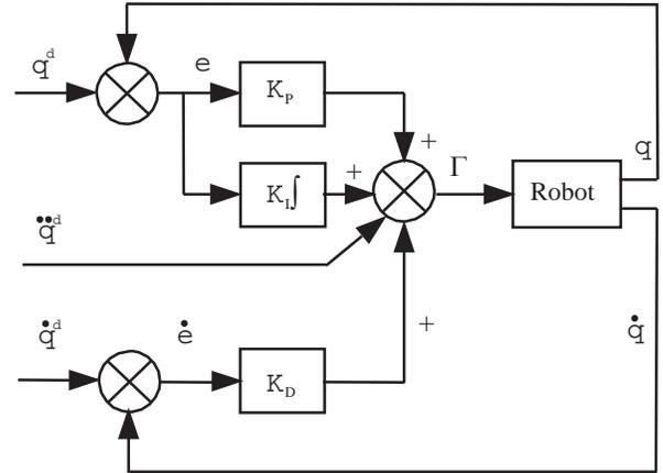
FIGURE 4. Control scheme of the Orthoglide 5-Axis
