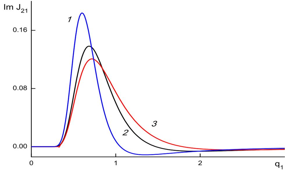
Fig. 6. Imaginary part of dimensionless density of longitudinal "crossed" current  $J_{21}$ ,  $\Omega_1 = 1, \Omega_2 = 0.5, q_2 = 0.1$ . Curves 1, 2, 3 correspond to values of dimensionless chemical potential  $\alpha = 2, 0, -5$ .
