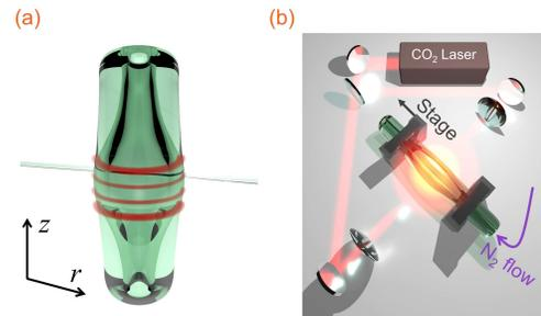
FIG. 1. (a) Bottle whispering gallery mode resonator. The red lines represent the mode light traveling in the resonator. (b) Schematic of the CO<sub>2</sub> laser bottle-like resonator fabrication setup.
