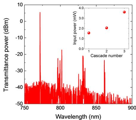
FIG. 5. Spectrum of cascaded Raman scattering. Pump light at 771.6 nm generates first-order Raman scattering around 802.0 nm, this generates the second-order around 831.2 nm and this generates the third-order around 861.3 nm.
