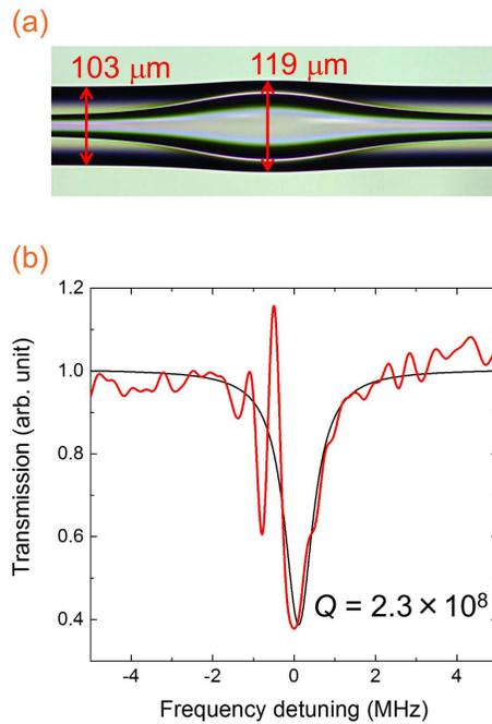
FIG. 2. (a) Microscope image of the hollow resonator. (b) Transmittance spectrum of a mode (red line) that was used for generating stimulated Raman scattering. The center wavelength of this mode is about 1545.09 nm. The transmission is normalized at the level of the laser background.  $Q$  is  $2.3 \times 10^8$  by Lorentzian fitting (black line).
