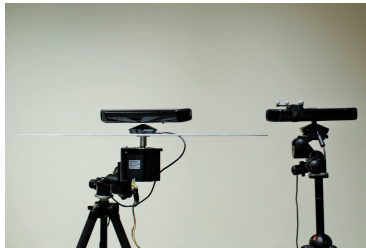
Figure 10: Multi-device interference experiment setup
