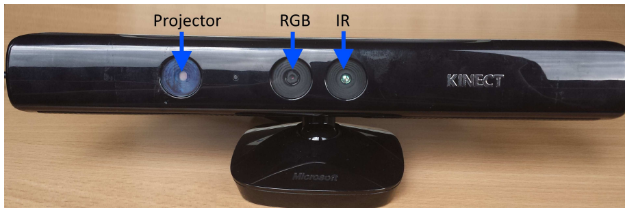
Figure 2: Sensor placement within a Kinect SL camera. The baseline is of approximately 7.5cm.
