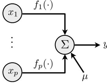
Fig. 1. Additive model diagram
