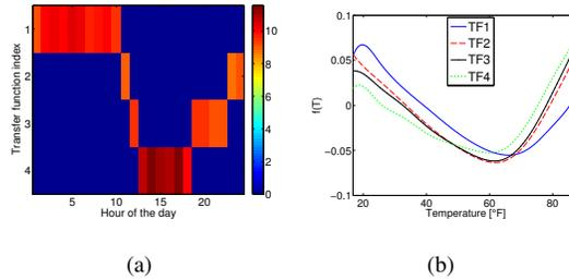
Fig. 8. Results on the GEFCom data with  $L = 4$ . (a)  $\mathbf{A}_{\text{temp}}$  matrix showing the activation of the temperature transfer functions for the 24 hours per day. (b) Shapes of the estimated temperature transfer functions.
