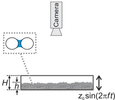
FIG. 1. (Color online) Schematic of the experimental set-up with definitions of the granular layer thickness  $h$  and the container height  $H$ . The magnified view of the wet granular sample illustrates a liquid bridge formed between two adjacent particles.  $z_0$ ,  $f$ , and  $t$  denote maximum vibration amplitude, frequency, and time in the laboratory frame correspondingly.
