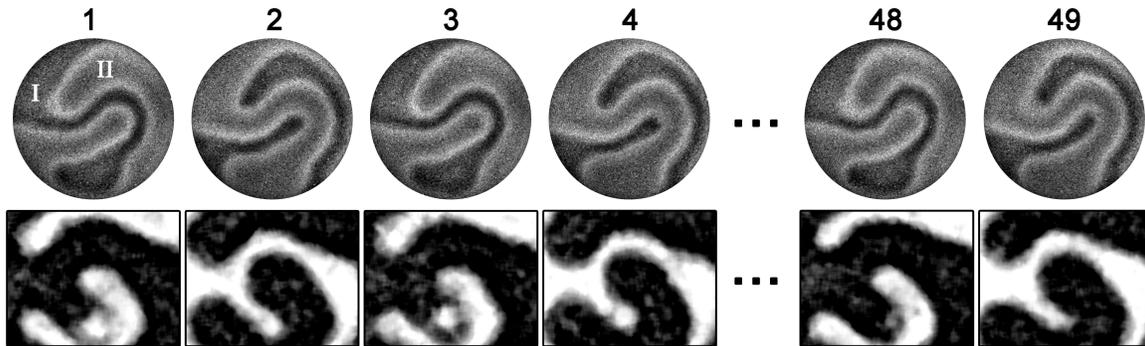
FIG. 3. Upper panel: Snapshots of a typical period doubling pattern taken at a fixed phase of consecutive vibration cycles (indicated as numbers) with  $f = 50$  Hz and  $\Gamma \approx 17.3$  g. Lower panel: Spatially resolved covariance of subsequent images captured as the granular layer collides with the container in another run of experiment with a closer view on the center region of the container. The brightness is related to the averaged mobility of the particles.
