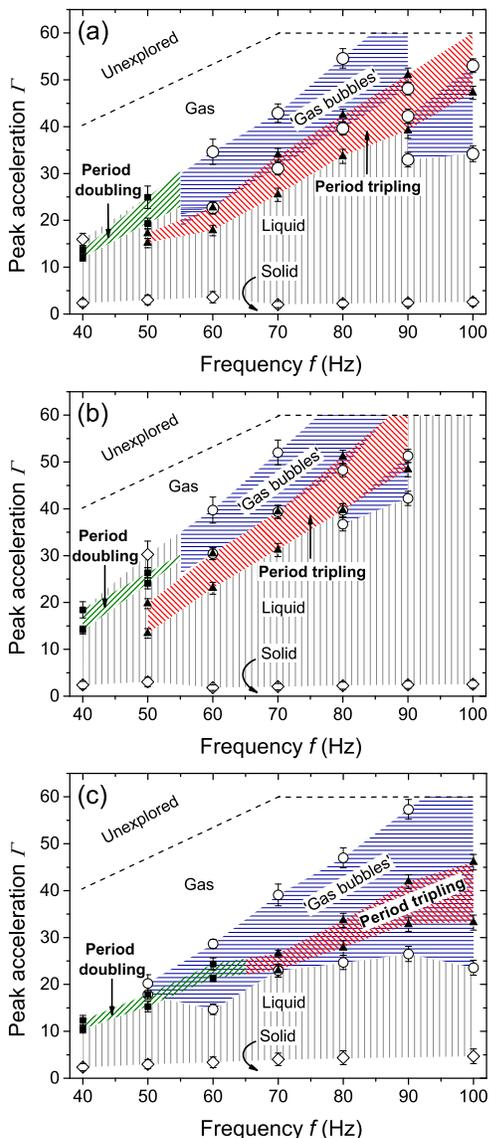
FIG. 4. (Color online) Stability diagrams for various combinations of sample mass  $m$  and container height  $H$  but the same filling fraction  $\Phi = 0.18$ : (a)  $m = 96$  g,  $h \approx 3.0$  mm and  $H = 10.6$  mm; (b)  $m = 111$  g,  $h \approx 3.5$  mm and  $H = 12.3$  mm; (c)  $m = 81.6$  g,  $h \approx 2.5$  mm and  $H = 9.0$  mm. The boundaries between various regimes are obtained the same way as in Fig. 2. Overlapping between various regimes corresponds to coexistence.
