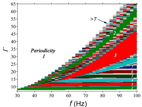
FIG. 6. (Color online) Periodicity predicted by the numerical analysis based on the single particle bouncing model. The parameters are chosen to match those in Fig. 2.
