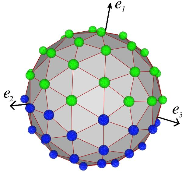
FIG. 1: (Color online) A snapshot of the Janus particle with wetting (blue atoms) and nonwetting (green atoms) hemispheres. The particle consists of 72 atoms rigidly fixed on vertices of a convex polyhedron (see text for details). Note that particle atoms are not drawn to scale. The unit vectors  $\mathbf{e}_1$ ,  $\mathbf{e}_2$  and  $\mathbf{e}_3$  form an orthonormal basis in a reference frame of the particle.
