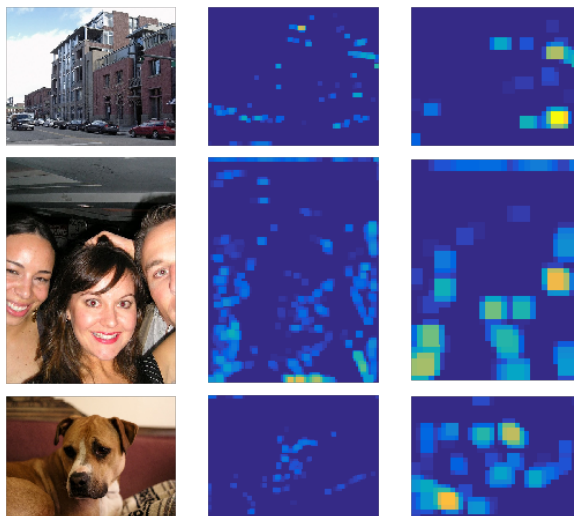
Figure 1: Convolutional feature responses at different image scales of two octaves apart. Different feature channels are visualized for each image. The responses are scale-selective, capturing different levels of contextual information. This phenomenon is studied and modeled in this work using scale volumes in order to obtain better object detection and localization performance.
