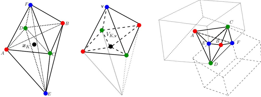
Fig. 4: Left: octahedral cell  $K$  for the CeVeFE-DDFV scheme. Center: illustration of  $V_{K,\mathbf{v}}$ . Right: construction of a degenerate octahedron from a non-conforming hexahedral mesh in a heterogeneous medium ( $CDEF$  is the intersection of the boundaries of two non-matching hexahedral cells).
