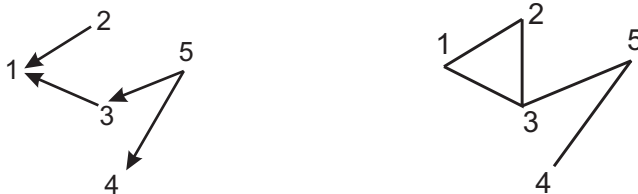
Figure 2: left: a small G_{\text{par}}^N with the three types of \mathbf{V} , with source node 5, transition node 3 and sink node 1; right: the induced concentration graph with an additional edge for (2,3) due to conditioning on the common sink node 1 of (2,3) .
