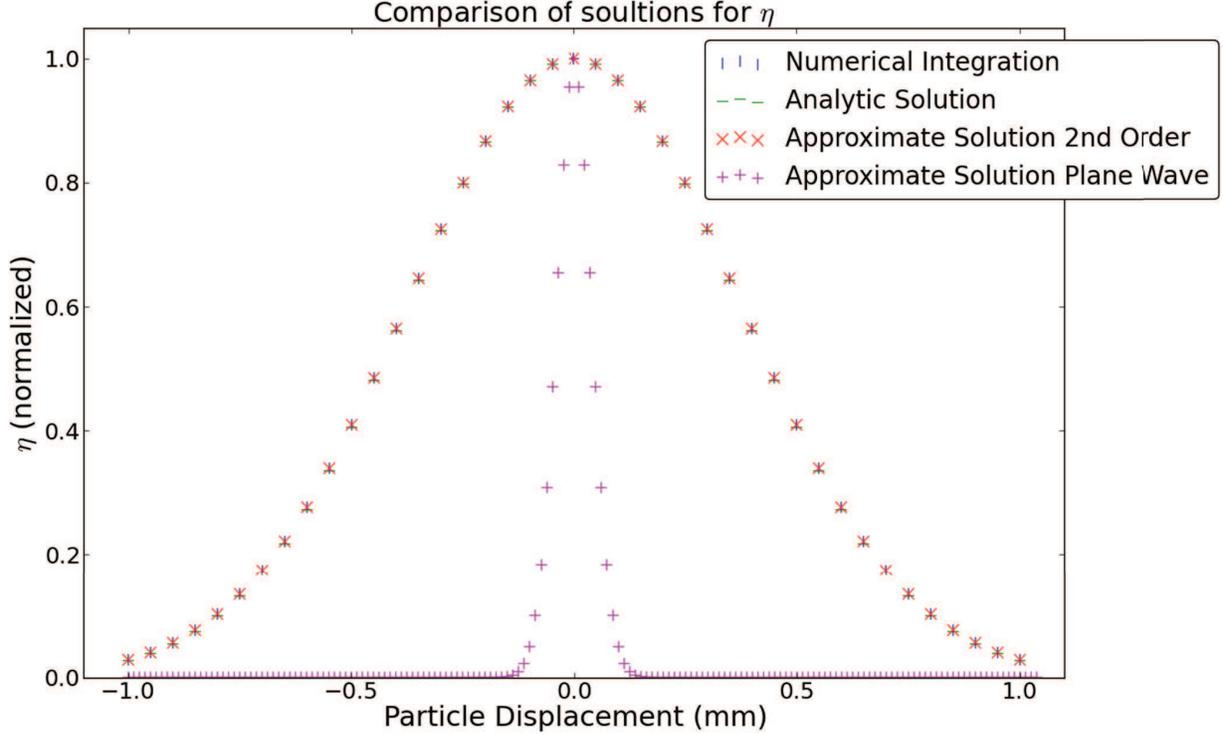
FIG. 3. Comparison of the coupling efficiency in water at  $g = 200$  mm and  $\lambda = 633$  nm, as calculated numerically on the plane of the lens, analytically evaluated on the plane containing the particle, and approximately integrated on the plane of the lens. We also show the result of evaluating with a plane wave approximation (neglecting  $h^2/2$ ) to demonstrate that this is an overapproximation.
