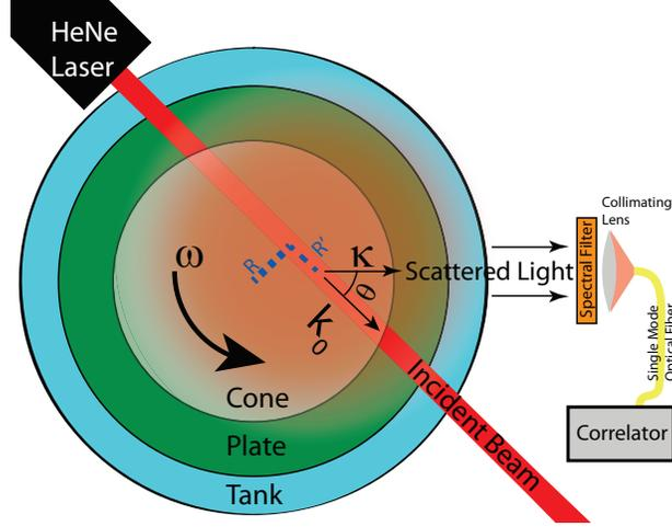
FIG. 1. System geometry top view. The incident beam scatters light over a wide angular range but only one scattering vector  $\vec{k}$  is collected by the single mode fiber via the collimating lens. The light output is fed into an avalanche photodiode photon counter, then the correlation card. The correlation yields the (time-averaged) shear rate  $s$ .
