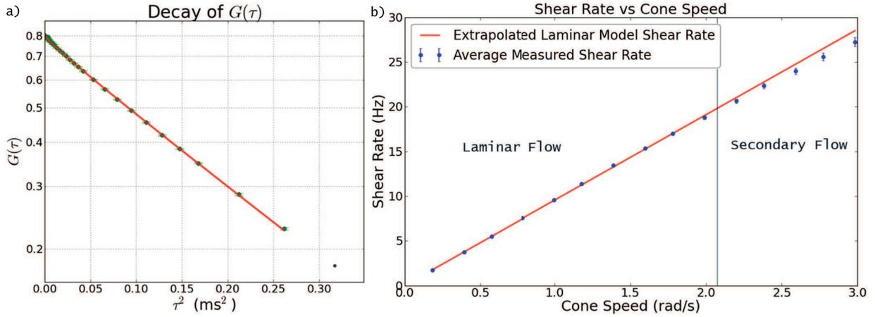
FIG. 2. a) Data and fit for a measurement taken at 0.4 rad/s cone speed at a scattering angle of  $20.5^\circ$ , with a  $2w_0 = 0.81 \text{ mm}$  beam and a  $2w_s = 1.05 \text{ mm}$  detector (on a logarithmic scale vs  $\tau^2$ , so  $G(\tau)$  is a straight line except near  $\tau^2 = 0$ ). b) The measured and theoretical shear rate as a function of cone speed at a scattering angle of  $20.5^\circ$  for a single run.
