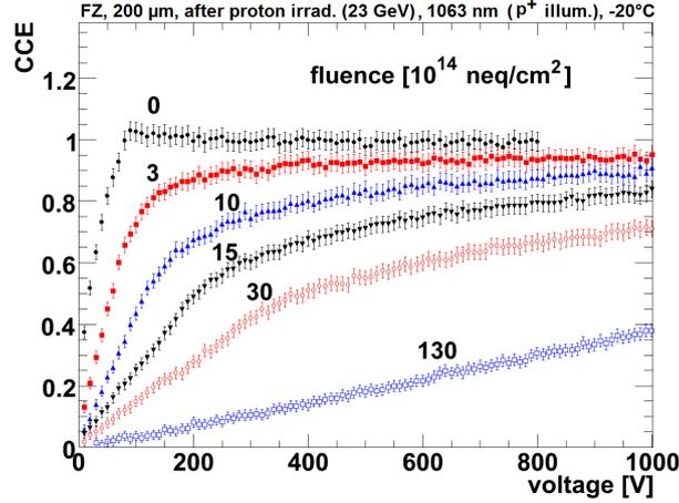
Figure 7: The CCE as a function of bias voltage for 200  $\mu\text{m}$  thick n-type sensors after irradiation with different fluences of 23 GeV protons. Laser light of 1062 nm wavelength was used to generate  $eh$ -pairs throughout the whole sensor depth.
