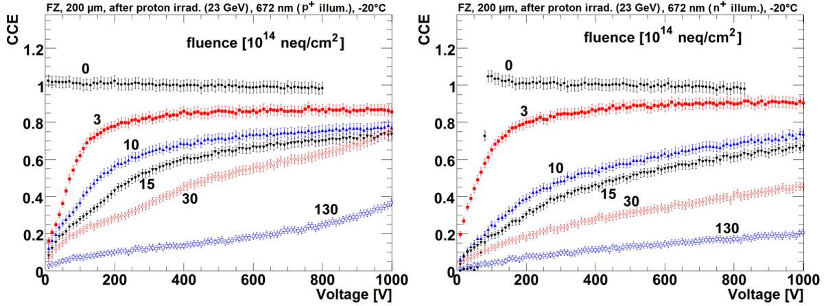
Figure 1: The CCE as a function of bias voltage is shown for 200  $\mu\text{m}$  thick n-type sensors after different fluences of 23 GeV proton irradiation. Laser light of 672 nm wavelength is used to generate  $eh$ -pairs close to the  $p^+$ -side (left), so that the signals are dominated by electron drift, or close to the  $n^+$ -side (right), so that the signal is dominated by hole drift.
