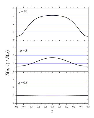
**Fig. 1.** Intensity of the NE concentration fluctuations S(q, z), relative to the value of the structure factor S(q), as a function of z for three wave numbers q. In the limit  $q \to 0$ , S(q, z) and S(q) become identical. The deviations increase with increasing q, but since the contributions for large q fall off as  $1/q^4$ , S(q) is a reasonable first approximation in practice.
