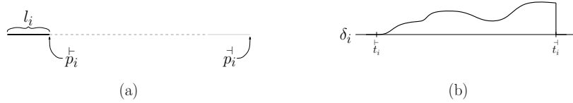
Fig. 1. (a) The physical specification of a vehicle v_i . (b) A possible speed profile, \delta_i , for a vehicle v_i .
