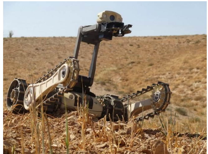
Fig. 1 - A Micro Tactical Ground Robot (MTGR) being tested on harsh terrain [3]
