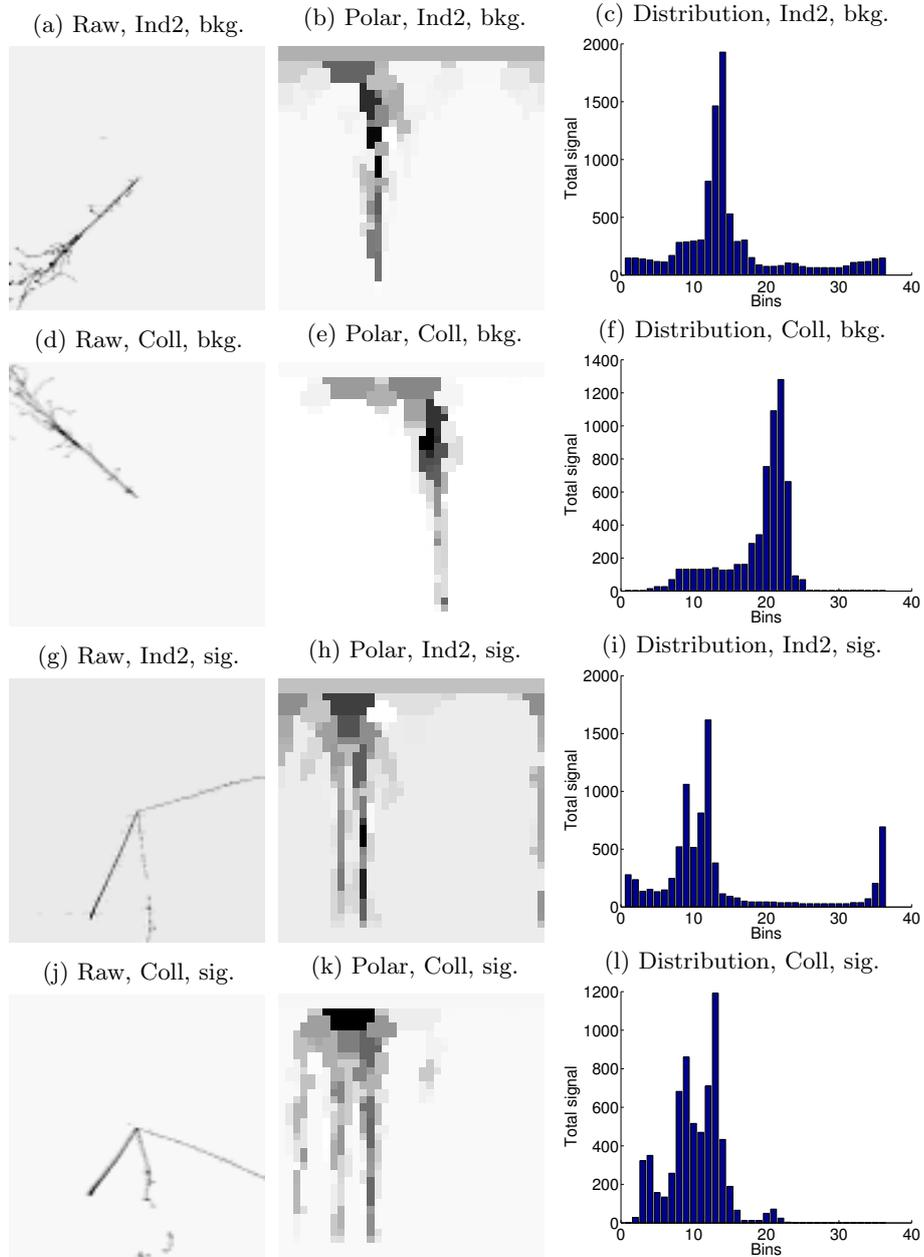
Fig. 1: The example of negative (bkg.) and positive (sig.) event presented in different perspectives, namely as a raw image observed in the detector, the image in polar coordinates, and charge distribution with 36 bins and radius equal 10 pixels. The each event is presented in Induction2 (Ind2) and Collection (Coll) views. Each row describes one event in a selected view.
