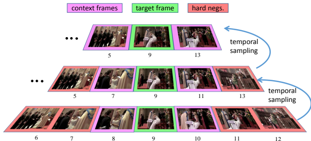
Figure 3. Multi-resolution sampling and hard negatives used in our full context model ( T = 1 ). For a target frame (green), we sample context frames (magenta) at varying resolutions, as shown by the rows in this figure. We take hard negatives as examples in the same video that fall outside the context window (red).
