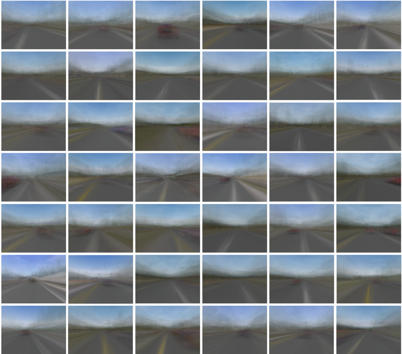
Figure 14: Activation pattern of neurons. For each of the 4096 neurons (42 shown here) in the first fully connected layer, we pick the top 100 images that activate the neuron most, and average them to get a activation pattern for this neuron. The neurons' activation patterns have strong correlation with the host car's heading, the location of the lane markings and traffic cars.
