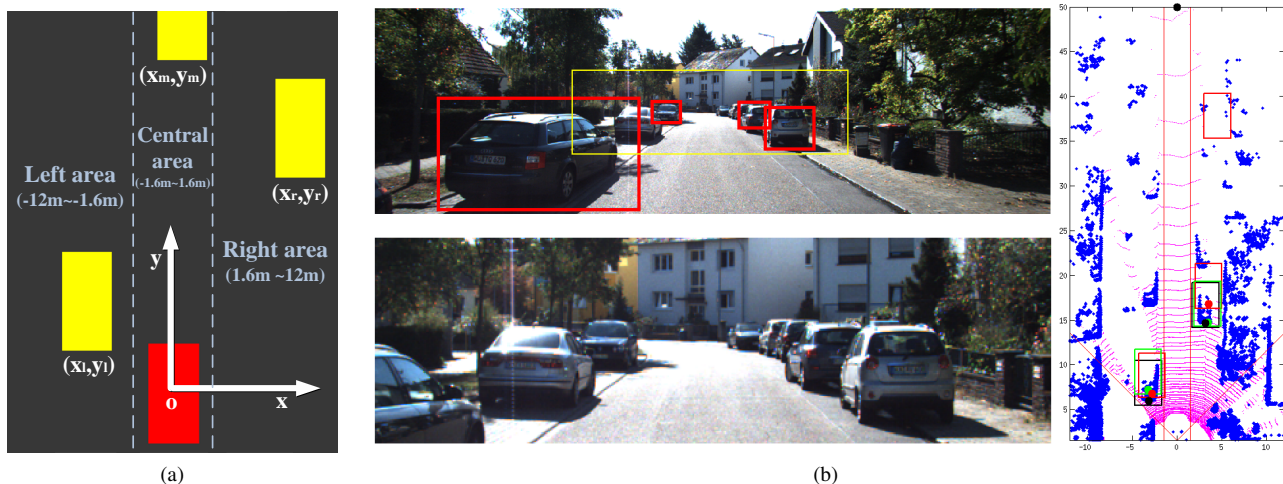
Figure 12: Car distance estimation on the KITTI dataset. (a) The coordinate system is defined relative to the host car. We partition the space into three areas, and the objective is to estimate the coordinate of the closest car in each area. (b) We compare our direct perception approach to the DPM-based mediated perception. The central crop of the KITTI image (indicated by the yellow box in the upper left image and shown in the lower left image) is sent to the far range CNN. The bounding boxes output by DPM are shown in red, as are its distance projections in the LiDAR visualization (right). The CNN outputs and ground truth are represented by green and black boxes, respectively.
