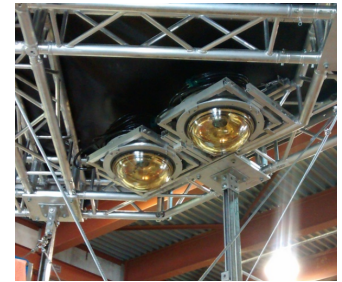
Figure 3: Two DOMs mounted at the top of the detector
