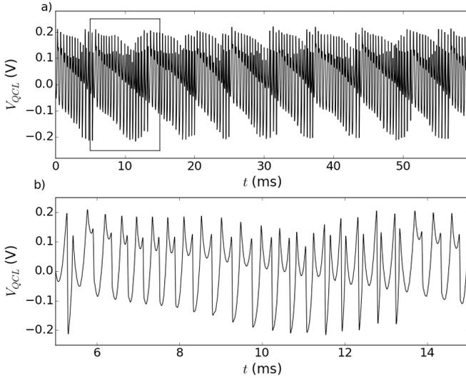
Fig. 7. (a) Representative oscilloscope trace of the voltage modulation detected at the QCL terminals (scope time base setting: 200 ms/div; sample rate: 2.5 MS/s). The SM waveform was obtained in response to forward translation of both oscillator and target ( $v_1 = 5$  mm/s and  $v_2 = 0.25$  mm/s). (b) Close up of the SM signal in panel (a) (highlighted region) showing the presence of the fringe sub-features.
