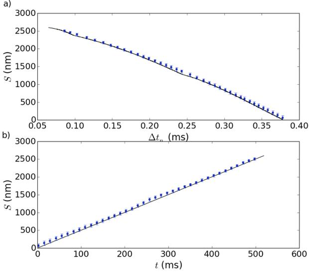
Fig. 5. Comparison between the theoretical displacement of the OT, represented by the solid lines, and the values obtained from Eq. (9) plotted with the corresponding error bars as a function of  $\Delta t_n$  (a) and  $t$  (b). Velocities set for the RT and the OT are, respectively,  $v_1 = 7$  mm/s and  $v_2 = 5$   $\mu$ m/s (only one point every 30 is drawn). The other parameters are as in Fig. 3.
