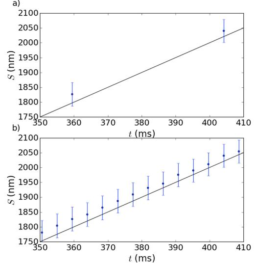
Fig. 6. Focus of  $S$  vs  $t$  in Fig. 5b for the same OT velocity and two different RT velocities:  $v_1 = 50$   $\mu\text{m/s}$  for the plot (a) and  $v_1 = 500$   $\mu\text{m/s}$  for the plot (b).
