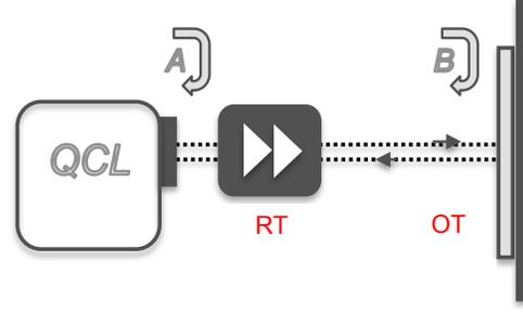
Fig. 1. Sketch of the common path sampling feedback interferometer.
