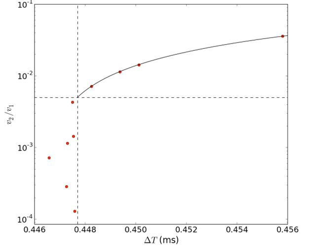
Fig. 4. Log-lin plot of the ratio  $v_2/v_1$  vs  $\Delta T$ . The solid line plots the hyperbolic relation predicted by Eq. (8), the red dots are the results of numerical simulations. The relation is satisfactorily verified down to  $v_2 = 30$   $\mu\text{m/s}$  (dashed line). The other parameters are as in Fig. 3.
