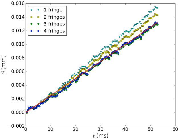
Fig. 8. Displacement  $S$  of the OT as derived by applying the formula (9) to the experimental data in Fig. 7 using interpolation on 1, 2, 3, 4 OT fringes (colored symbols). The red line indicates the imposed OT translation  $S_{\text{exp}} = v_2 t$ .
