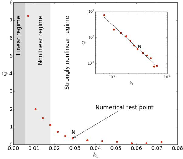
Fig. 2. Plot of the ratio  $Q$  between the amplitude of the frequency peak at  $\omega_1$  and that of the frequency peak at  $\omega_1 - \omega_2$  versus the feedback coefficient  $k_1$  ( $k_1/k_2 = 1.18$ ). The two target velocities are  $v_1 = 7$  mm/s and  $v_2 = 0.25$  mm/s. Inset: log plot of  $Q$  vs  $k_1$  in the “nonlinear” and “strongly nonlinear” regime. The solid line represents the best fit  $Q \propto k_1^{-1.98}$ .
