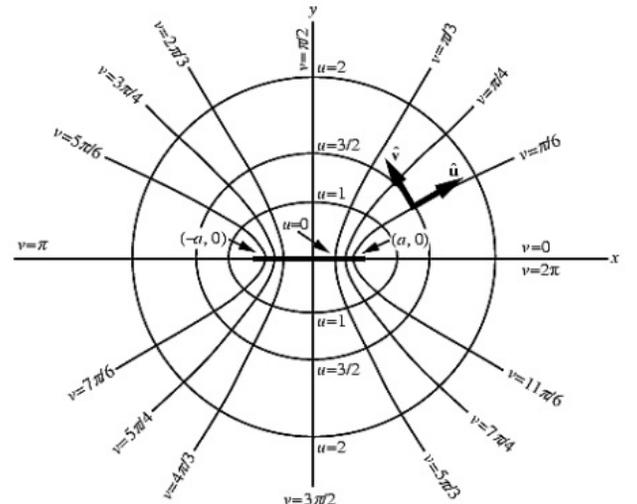
Figure 2. Elliptic cylindrical coordinates.
