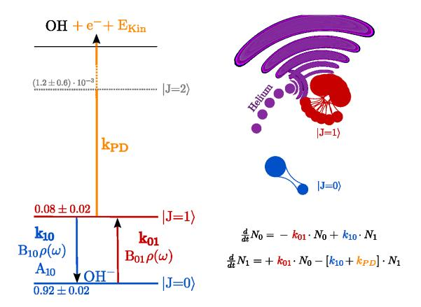
Figure 1: OH<sup>-</sup> rotational energy levels and coupling rates
