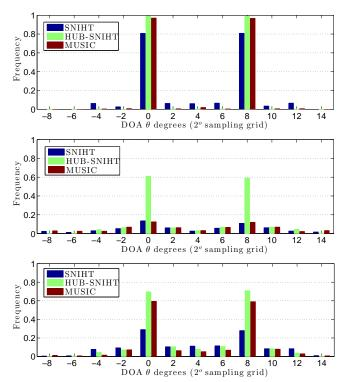
Fig. 1. Bar plots of relative frequency of DOA estimates. Two equal power independent Gaussian sources arrive from DOA  $0^o$  and  $8^o$  and the noise has i.i.d. elements from IG-CG distribution with unit variance and shape  $\lambda=0.1$ . SNR =-10 dB and Q=50 (upper plot), SNR =-20 dB and Q=50 (middle plot) and SNR =-10 dB and Q=50 (lower plot).
