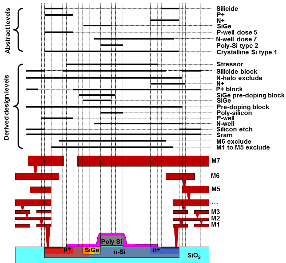
Fig. 4 Example of level generation. The designer draws shapes on abstract levels (top) which have a direct correspondence with the relevant parameters. Those layers are drawn irrespectively of design rules. For example, high-doping levels (N+ and P+) can be drawn with edges coincident with the silicon pattern. In a later data-preparation step, these layers are translated in counter-intuitive design levels (bottom) and the design rules are enforced.
