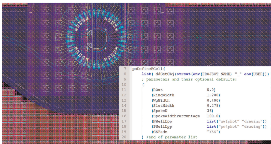
Fig. 3 Definition and representation of the pCell of a spoke-ring modulator
