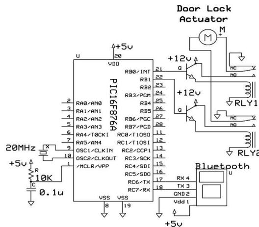
Fig. 16. Schematic of Car Door Lock System
