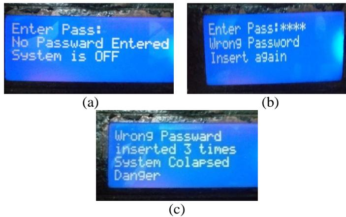
Fig. 4. LCD Output of the Security System
