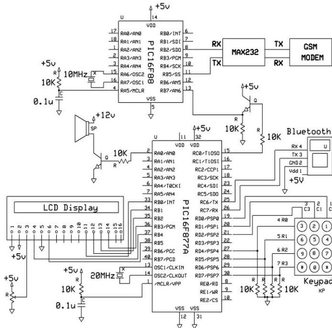
Fig. 3. Hardware Section for Primary Security
