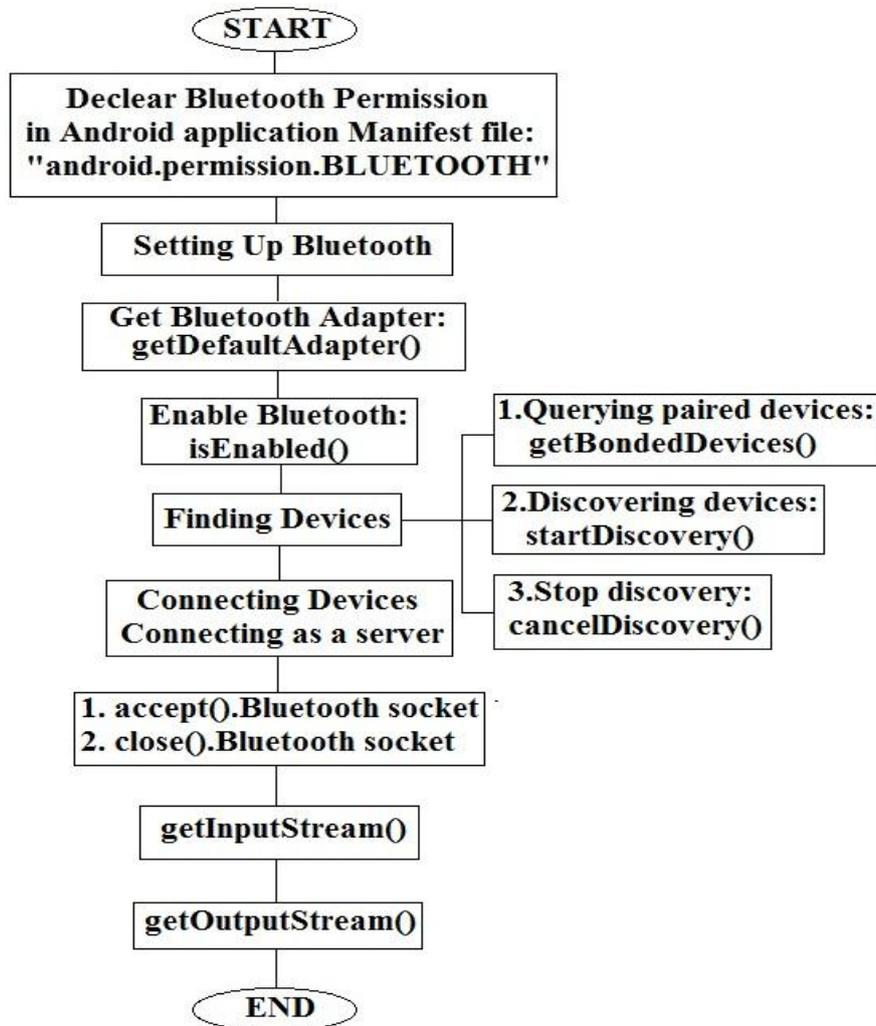
Fig. 1. Android-Bluetooth Communication Flow
