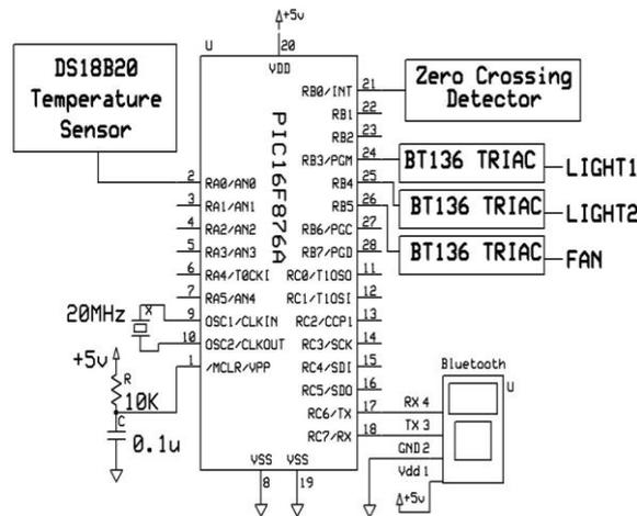
Fig. 9. Schematic for Home Appliance System
