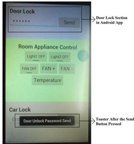
Fig. 7. Android App Door Lock Section
