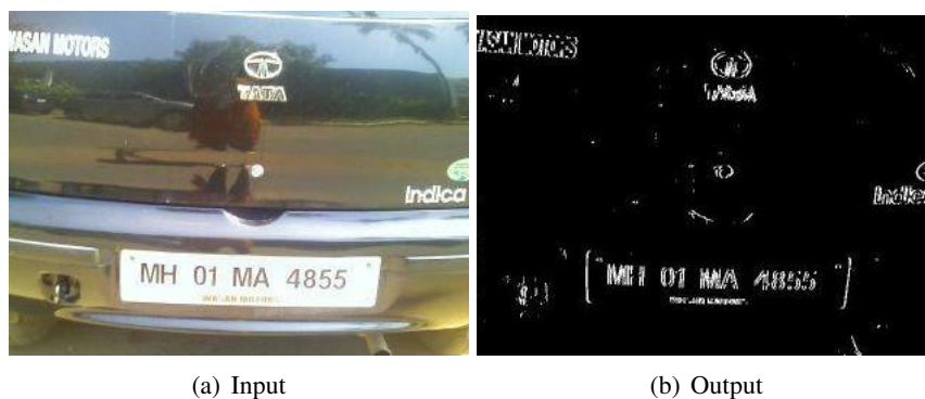
Figure 5: Sample vertical edge output
