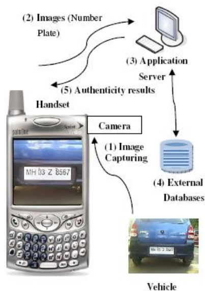
Figure 1: The high-level client-server architecture of the solution.
