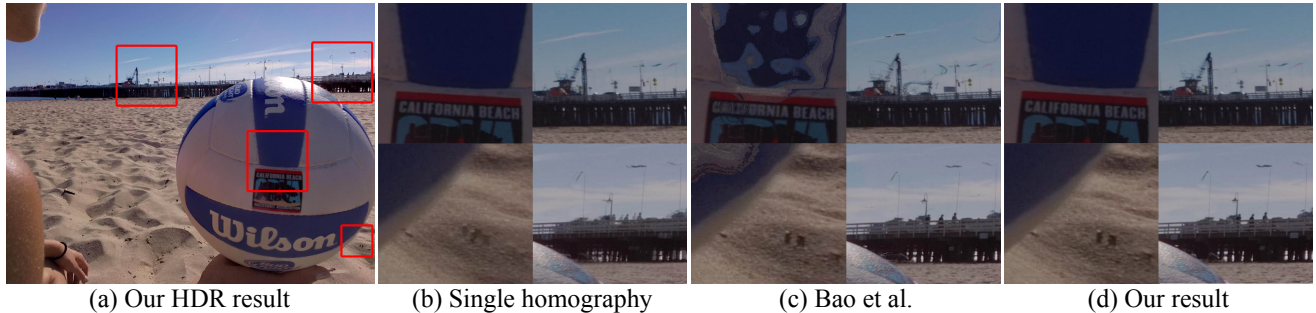
Figure 1: When capturing HDR stacks without a tripod, parallax and non-rigid scene changes are the main sources of artifacts. The picture in (a) is an HDR image generated by our algorithm from a stack of two pictures taken with a hand-held camera (notice that the volleyball is hand-held as well). A common and efficient method to register the images is to use a single homography, but parallax will still cause ghosting artifacts, see (b). One can then resort to non-rigid registration methods; here we use the fastest method of which we are aware, but artifacts due to erroneous registration are still visible (c). Our method is several times faster and, for scenes with parallax and small non-rigid displacements, produces better results (d).
