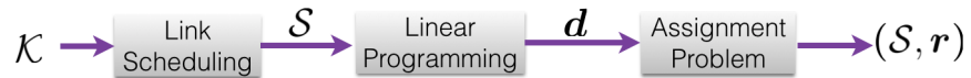
Fig. 4: The separated solution with a heuristic link scheduling and assignment-inspired power control, where the optimal GDoF tuple is obtained via linear programming over the selected convex polytope.
