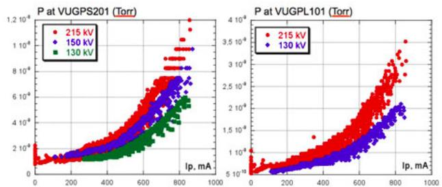
**Figure 2.** Variation of the vacuum pressure in the arcs as a function of RF cavity voltage. The reduction of RF High Voltage results in a slower growth of the dynamical vacuum pressure because the induced lengthening of the beam bunch reduces the charge density with same total beam current and thus the e-cloud acceleration towards the beam line is weaker.
