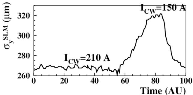
**Figure 3.** Effect of the CW sextupoles on the transverse dimensions of the positron beam. When the CW sextupole current is lowered from 210 A to 150 A, a sizeable growth of vertical beam size is observed at the Synchrotron Light Monitor from 265  $\mu\text{m}$  to 320  $\mu\text{m}$ .
