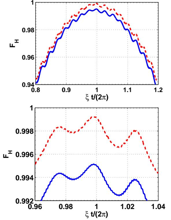
FIG. 2. Fidelity dynamics of the Hadamard gate as a function of  $\xi t/(2\pi)$  with the initial state of the polariton qubit being  $|+\rangle$ , where the red dashed and blue lines being plotted without and with decoherence, respectively.
