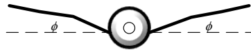
Figure 4. Auxiliary diagram of the flapping motion with the definition of the flapping angle. View in the direction of the flow.
