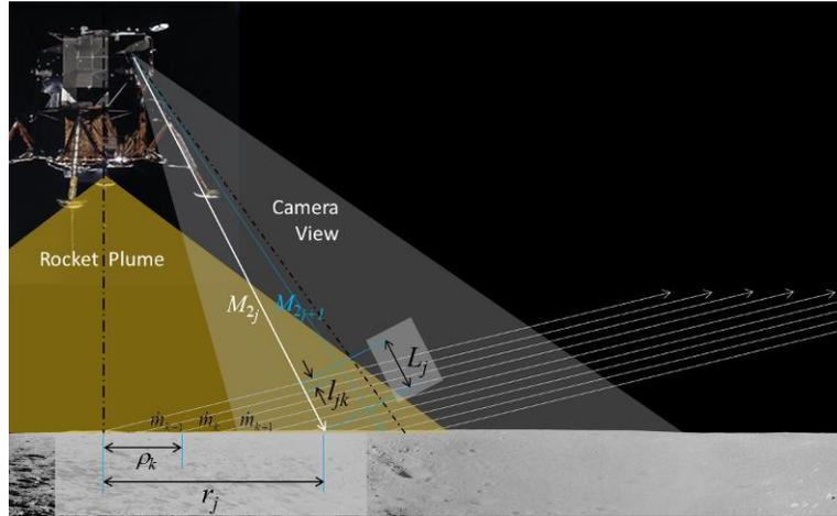
Fig. 13. Schematic diagram of erosion model geometry, leading to  $\varphi = 2$  in Equation (4).
