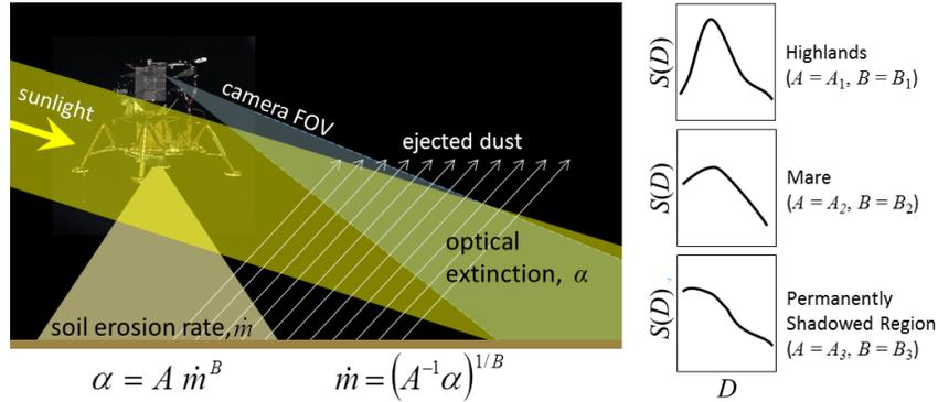
Fig. 2. Optical measurement of dust erosion rate is affected by the local soil size distribution  $S(D)$ . Note that  $A$  and  $B$  are found from  $S(D)$  associated with soil properties at a specific region on the lunar surface, as well as the properties of the gas exiting the rocket nozzle used to generate  $v(D)$ , based on the specific engine design.
