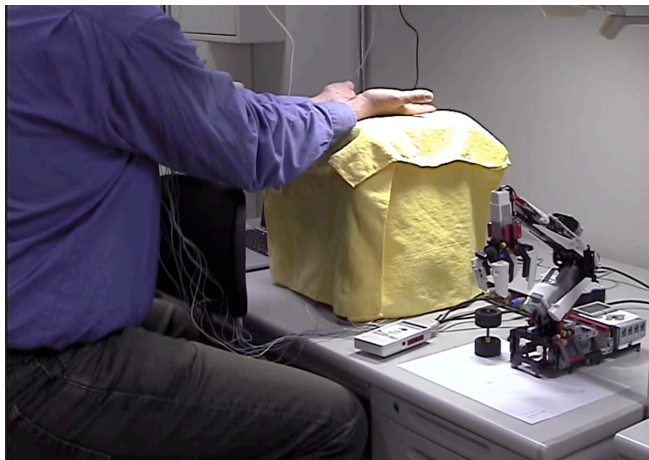
Figure 1. The autdBCI user with hands placed under the AUTD device and operating mentally the small six commands-based robot placed on the right side.
